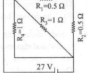
**60.** Find the voltage and current passing through the resistor R<sub>2</sub> shown in the following circuit
